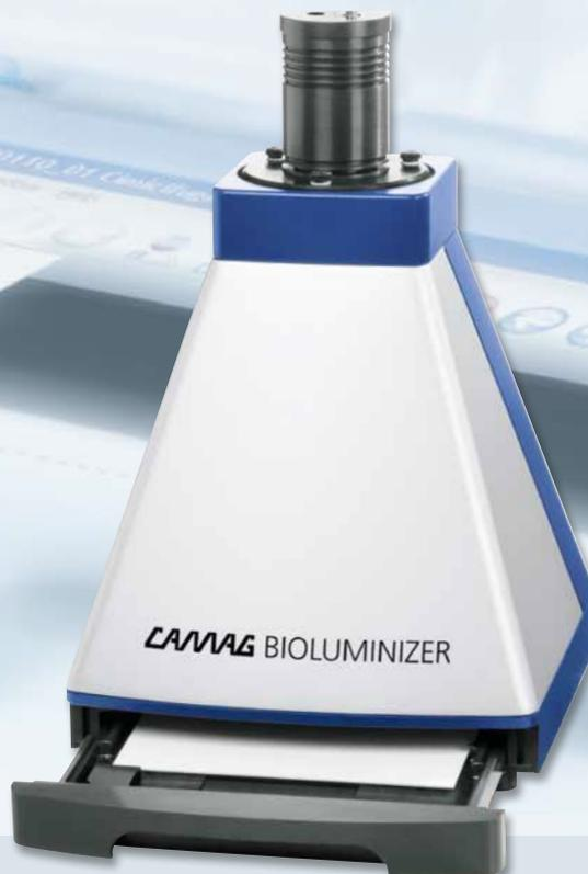
The Bioluminizer system is consisting of a compartment excluding any extraneous light, climate controlled for extended stability of the plate, and a 16 bit CCD digital camera of high resolution and high quantum efficiency. It features ergonomic design and easy, intuitive handling in stand-alone mode using the special software.
