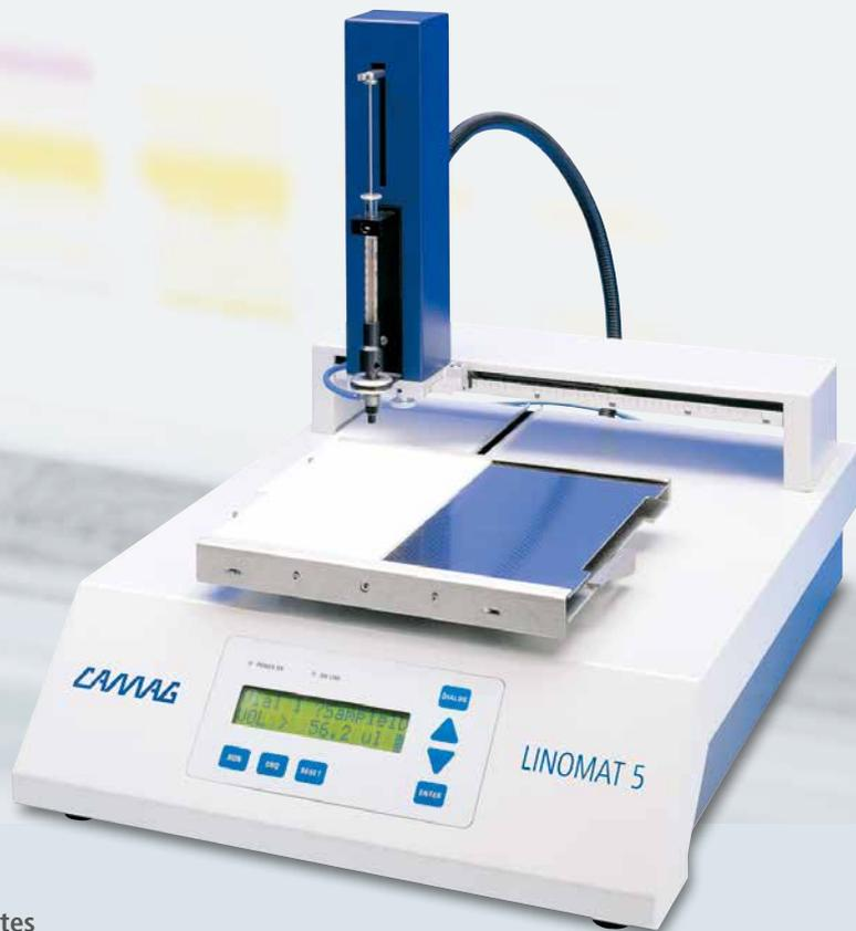
With the Linomat 5 samples are sprayed onto TLC/HPTLC plates in the form of bands with nitrogen or compressed air. Sample application is automatic, only changing the syringe (filling, inserting and rinsing) is manual. The Linomat is suitable for routine use.
